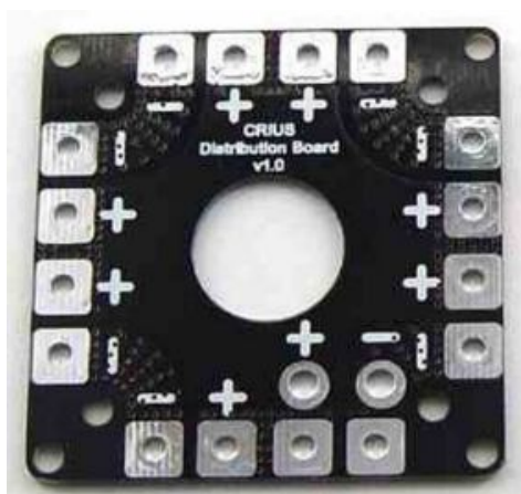
Figure 12 power distribution board
