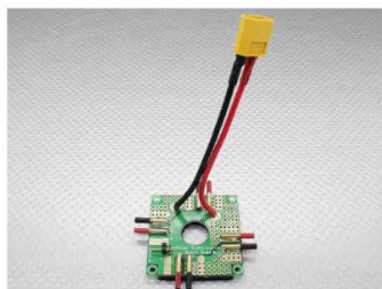
Figure 13 power distribution board
